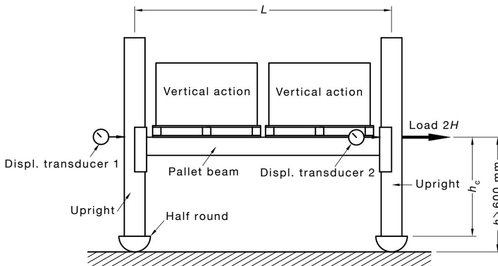
FIGURE 7.5.2.3 PORTAL TEST SET-UP
