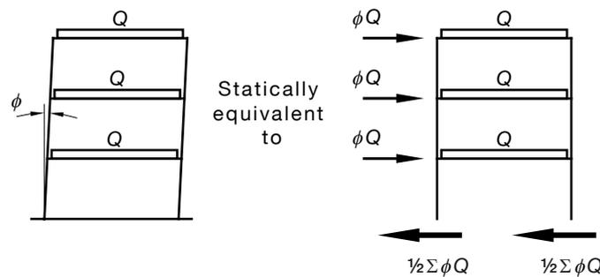
FIGURE 3.3.2.1 EQUIVALENT HORIZONTAL FORCES
