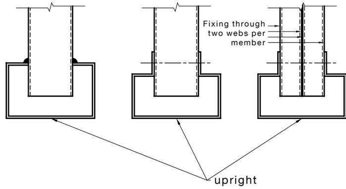
(a) Connections with large warping restraint
