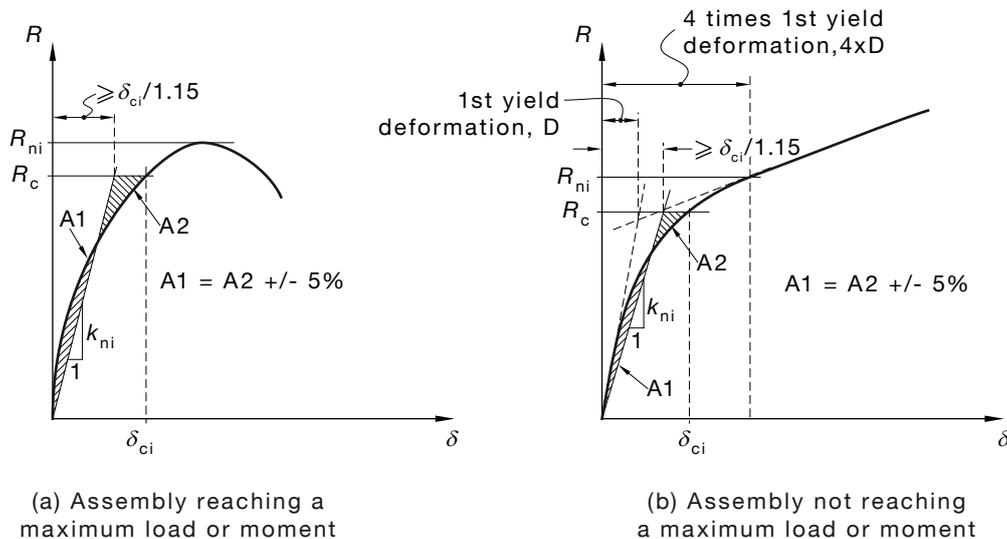
FIGURE 7.2.2.2 DERIVATION OF AN ASSEMBLY STIFFNESS
