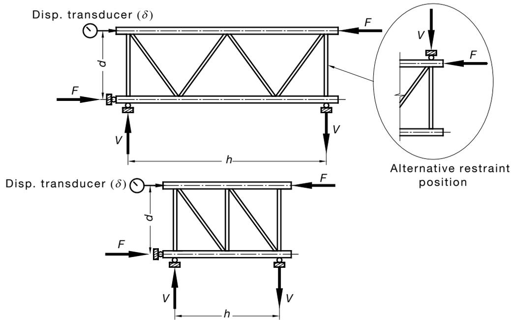
FIGURE 7.7.1.2 TEST ARRANGEMENTS FOR MEASURING THE SHEAR STIFFNESS OF BRACED FRAMES
