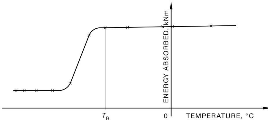
FIGURE 7.10.3(a) CHANGE OF TRANSITION TEMPERATURE ( $T_R$ )
