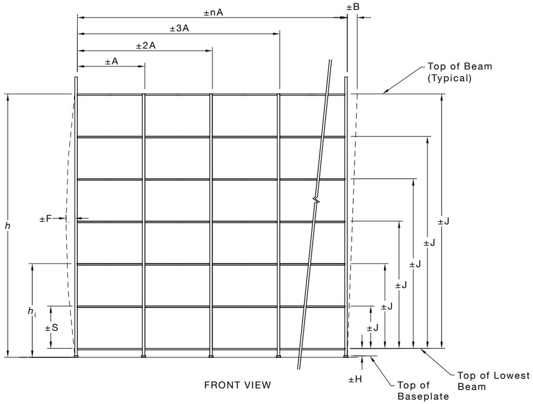
(a) Down-aisle tolerances (closed face racking)
