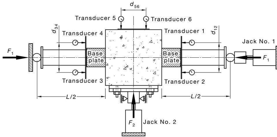
FIGURE 7.9.2(a) TEST ARRANGEMENT FOR FLOOR CONNECTIONS (PLAN)
