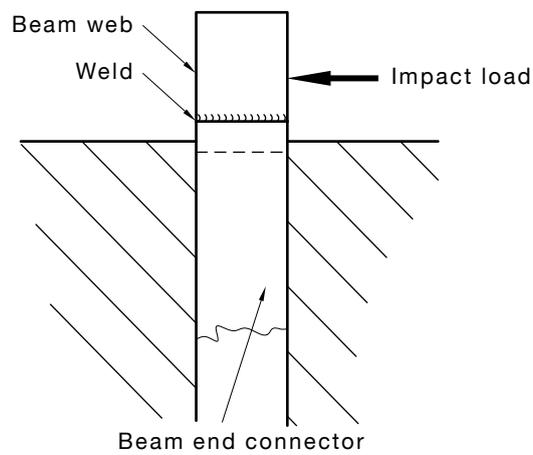
FIGURE 7.10.2(c) TEST ARRANGEMENT OF THE WELD BETWEEN BEAM AND CONNECTOR
