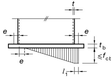
FIGURE 6.3.2.3 EFFECTIVE BEARING LENGTH AND LENGTH OF PLATEAU AT CONSTANT CONTACT PRESSURE
