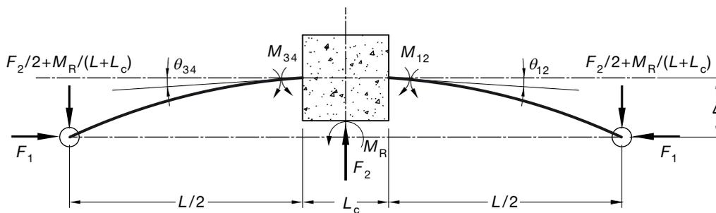
FIGURE 7.9.3 FORCES AND DEFLECTIONS IN THE TEST ON FLOOR CONNECTIONS
