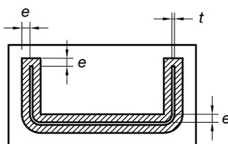
FIGURE 6.3.2.1 EFFECTIVE AREA OF THE BASE PLATE
