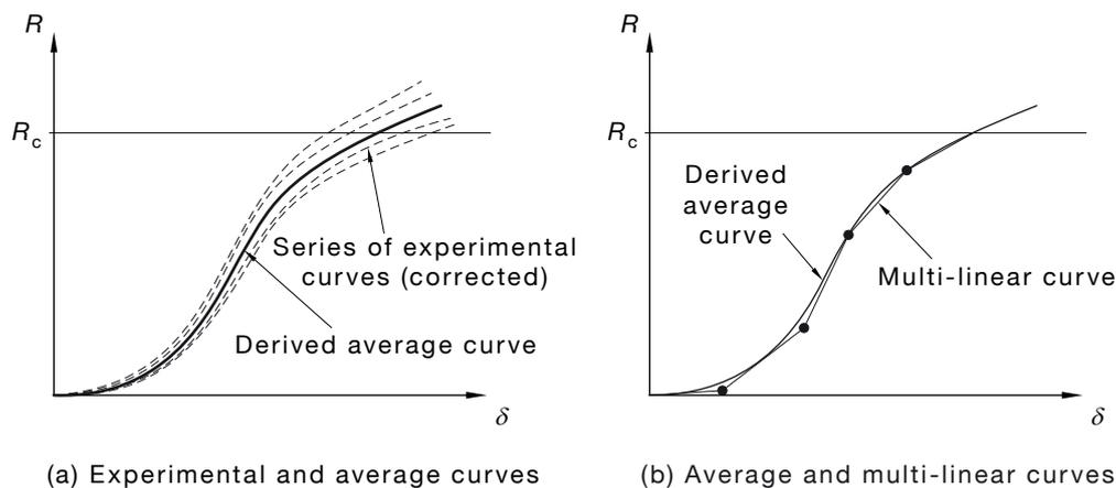
FIGURE 7.2.2.3 DERIVATION OF A MULTI-LINEAR CURVE
