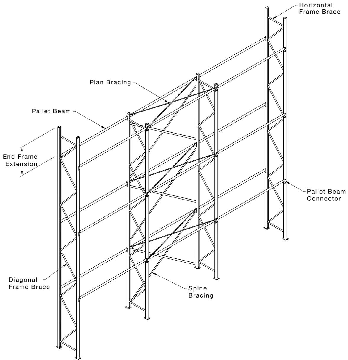
(b) Braced closed-face racking
