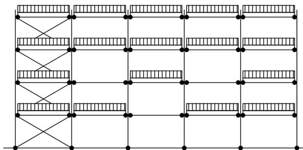
b) Typical loading pattern for a braced rack
