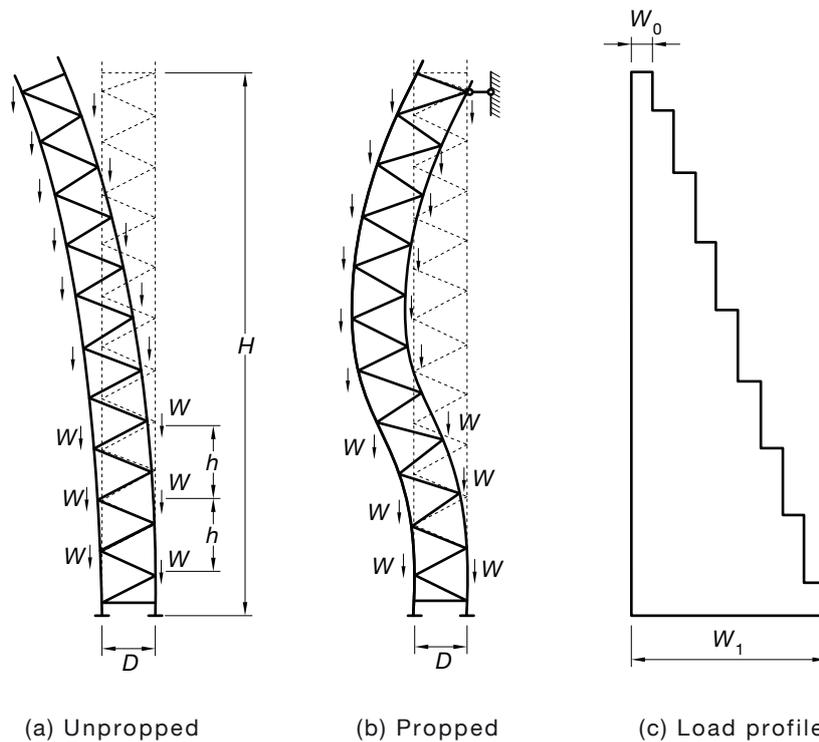
FIGURE C2 ASSUMPTION FOR SIMPLIFIED CROSS-AISLE STABILITY ANALYSIS
