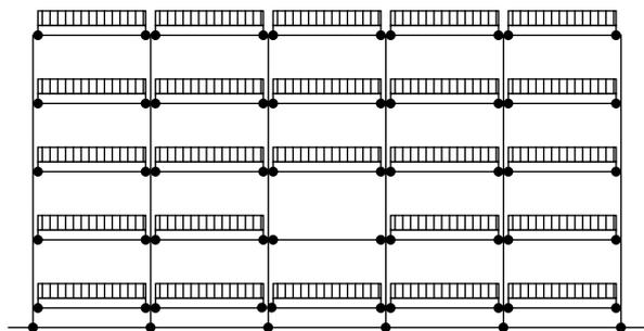
c) Additional loading pattern when the lowest beam is near the ground
