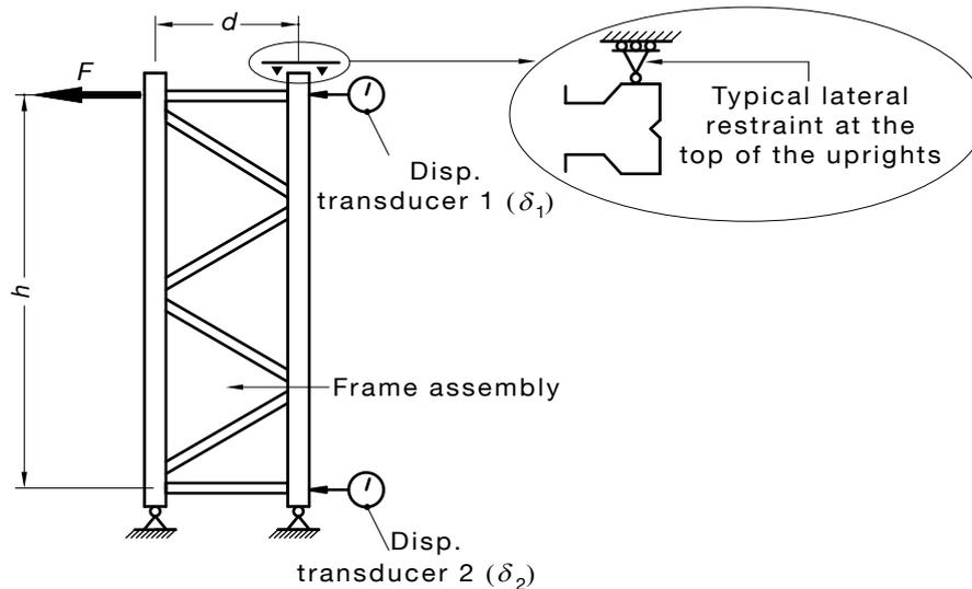
FIGURE 7.7.2.3 TEST ARRANGEMENTS FOR MEASURING THE COMBINED BENDING AND SHEAR STIFFNESS OF BRACED FRAMES
