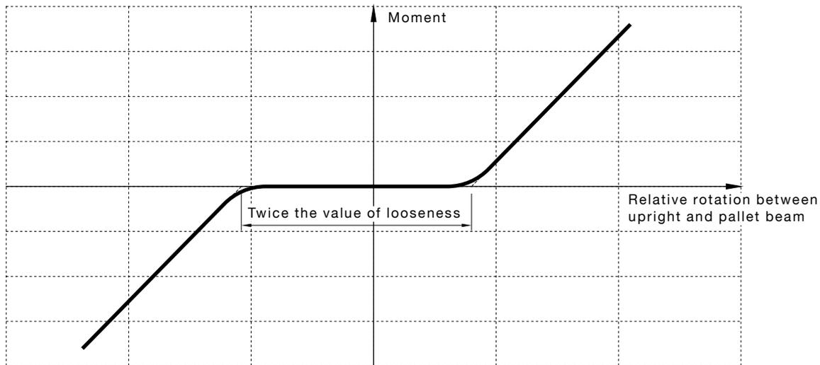
FIGURE 7.5.3.3 CANTILEVER RESULTS FOR CONNECTOR LOOSENESS DETERMINATION
