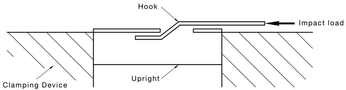
FIGURE 7.10.2(b) TEST ARRANGEMENT OF A SINGLE HOOK BETWEEN BEAM AND CONNECTOR
