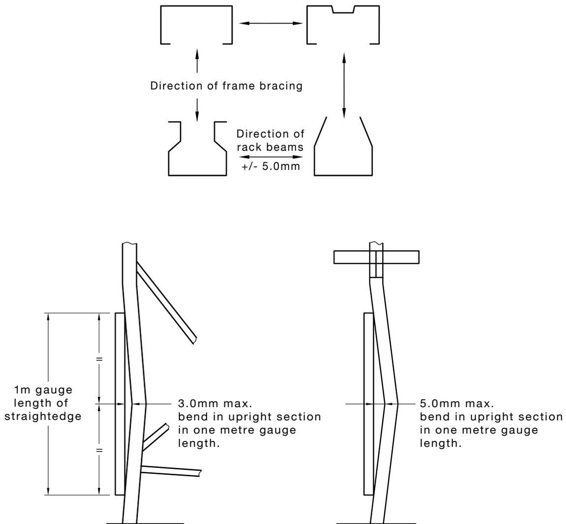
FIGURE 8.3.2 TYPICAL UPRIGHT SECTIONS AND METHOD OF MEASUREMENT
