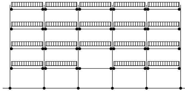
a) Typical loading pattern for an unbraced rack
