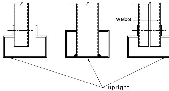
(b) Connections with partial warping restraint
