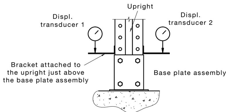
FIGURE 7.9.2(b) APPROPRIATE POSITIONS FOR TRANSDUCERS
